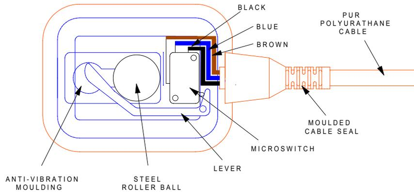
The micro-switch assembly inside the float, axially mounted in line with the weight, changes contacts according to the float's position, as in the diagram below. Therefore as the liquid level drops or rises slowly, a pump or flow control suitably connected, can be switched in or out to maintain an average level of the liquid. By connecting only one side of the switch, the unit can be also used to fill or empty the tank as required.
